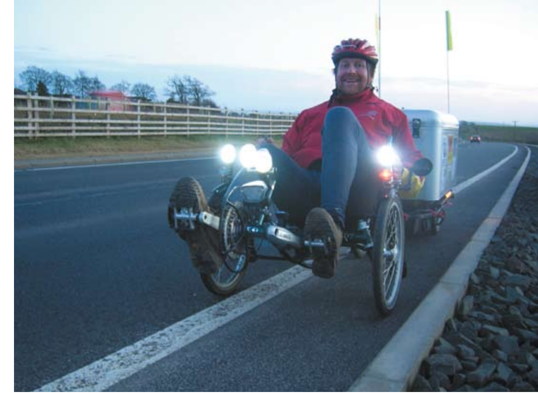
ABOVE: Dynamo hubs and solar panels fuel the LED lighting system
